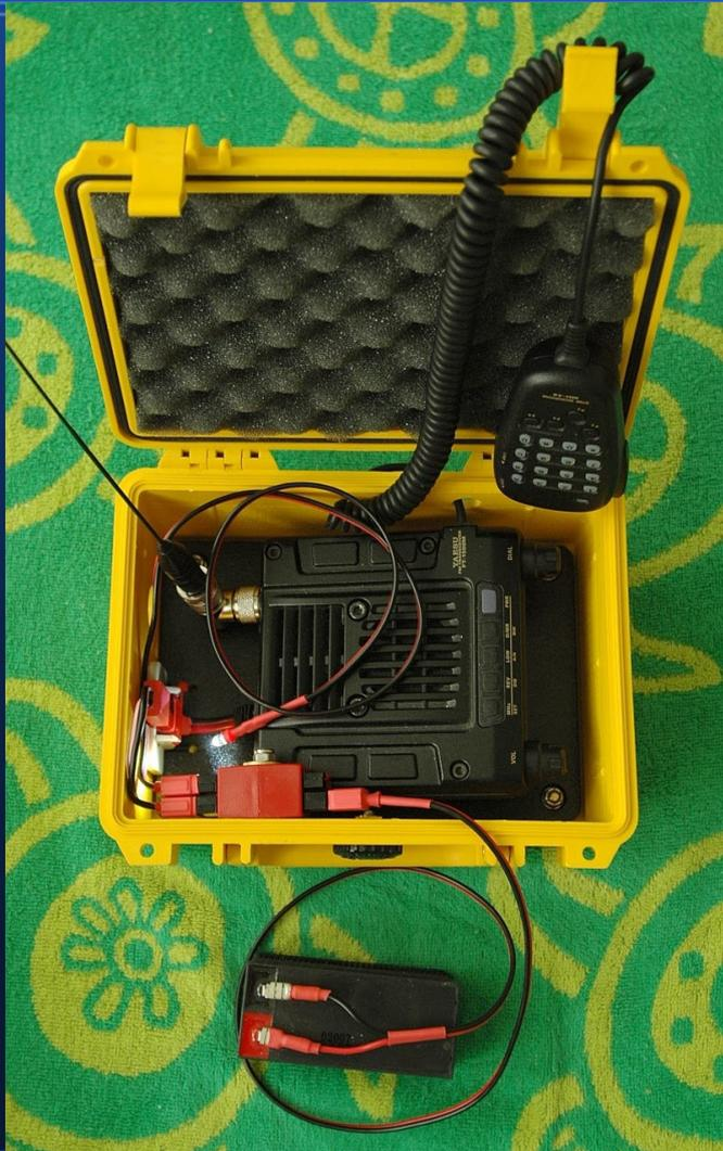
The mobile rig is mounted with the front tilted up such that the display can be seen better
