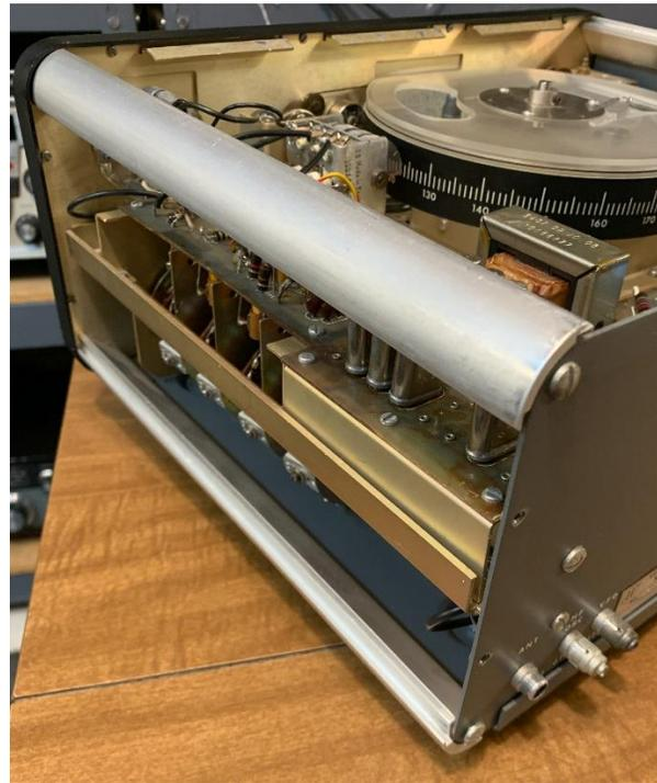
Right Rear View with the Top Panel and Right-Side Panel removed. Note open Side Panel mounting screw holes visible on the rear panel.
