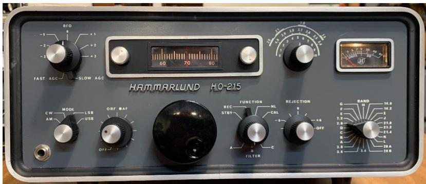
The front panel is conveniently laid out and is somewhat reminiscent of the Collins 75S-3C on which its design is based. Reviewing the important controls, one can see the prominent main tuning knob. It is nice to see that this radio uses generally available open stock
