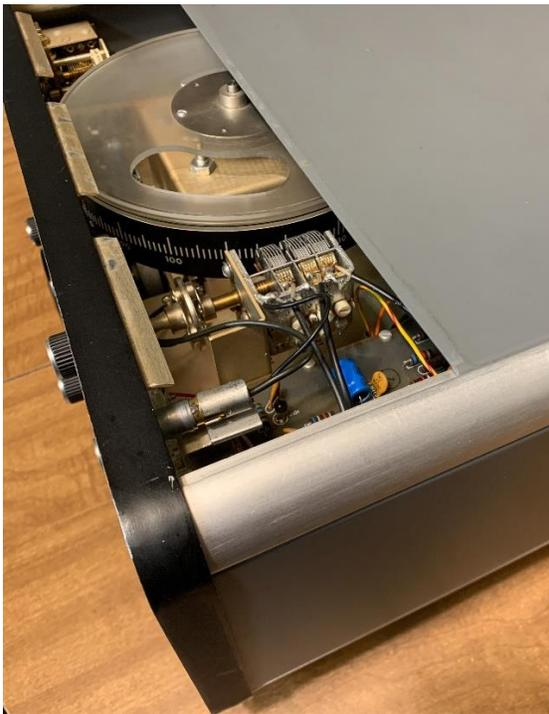
Right Front Corner view with the Top Cover pulled back a few inches. See how the Panel slides into the right upper extrusion.
