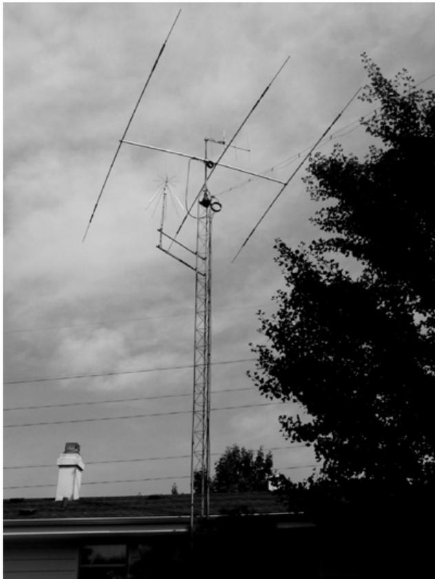
**Bill has an impressive antenna tree sprouting a 3 element multiband HF beam, discone, 2 meter beam and multiband B&W sloper.**
