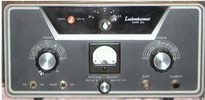
The matching Hallicrafters HT-45 Loudenboomer Mark IIA Linear Amplifier. A Story for a future installment. Not shown is Model P-45, 3,000 (VDC) Power Supply.
