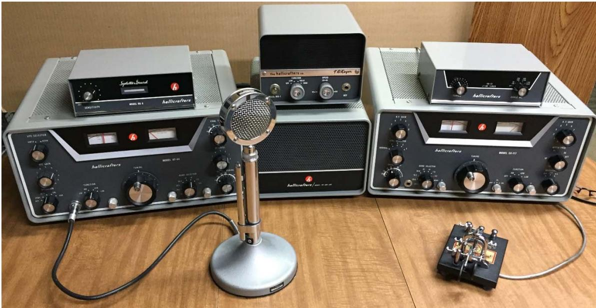
**HT-44 Transmitter with the HA-8 Splatter Guard on top, PS-150-120 Speaker/Power Supply with the HA-1 'TO Keyer on top, SX-117 Receiver with the HA-10 LF/MF Tuner on top. Also, see the Astatic D-104 Microphone and Vibroplex VibroKeyer**
