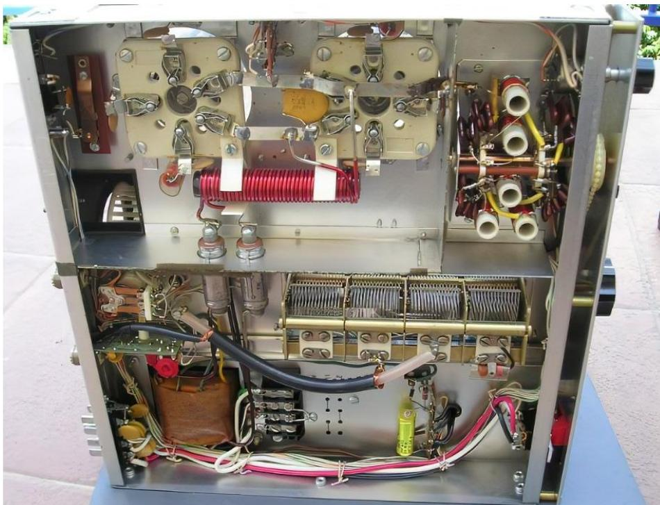
**Drake L-4B Linear Amplifier – Bottom Interior View
