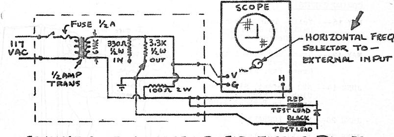
SCHEMATIC OF AN ADAPTER FOR TESTING DIODES TRANSISTORS - CAPACITORS ETC. IN CIRCUIT OR OUT OF
