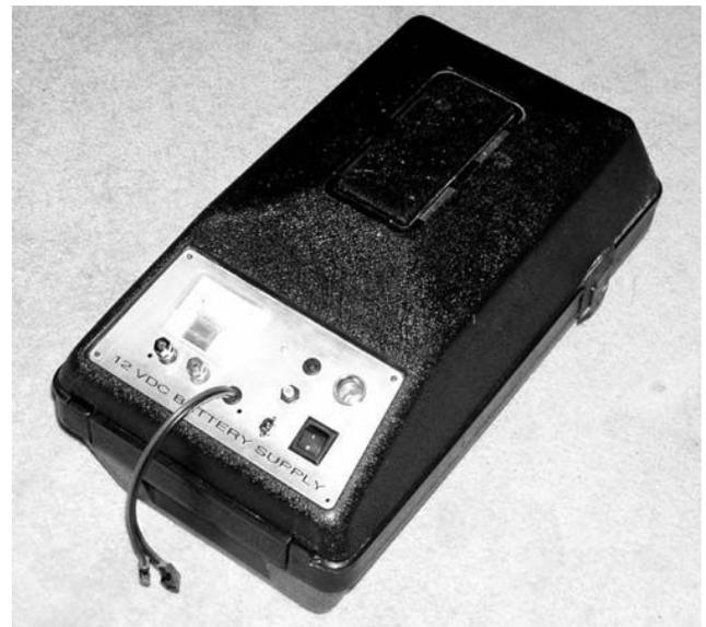
The exterior of the 12 VDC Battery Supply shows the voltmeter, circuit breaker, switch and power termination's
