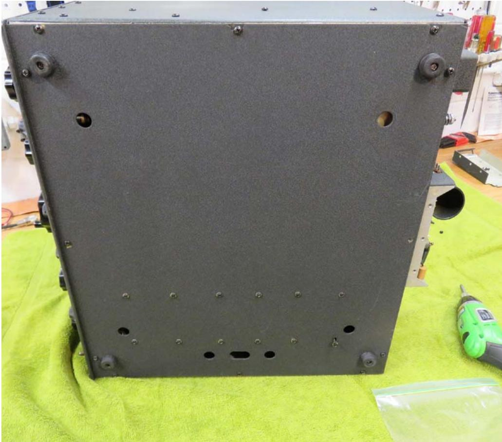
Next the bottom cover is removed. It is held on by a total of 24 screws!
