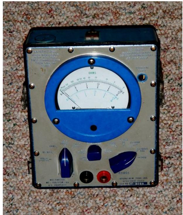
(VOM). These are the most rugged and most accurate (3-5%) VOM's ever made. Checking on the internet you will find they sell reconditioned for from \$99 to \$149.
