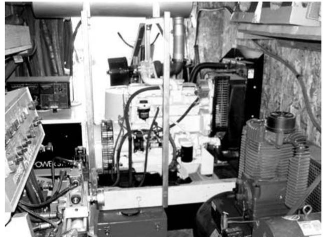
We again had the benefit of central “portable power” from the trailer mounted 50 kW generator provided by Ed Frac, AA9WW.
