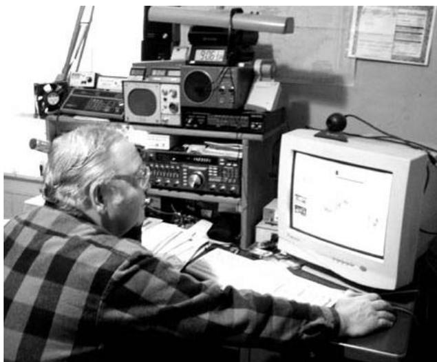
**Terry is shown here operating SSTV. Note the rig-PC interface consists of the PC audio mic in front of the transceiver speaker and to transmit, he holds the transceiver mic in front of the PC speaker.**
