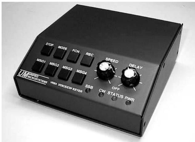
This console "keyer" by W9XT can be interfaced with the PC for ease in "contesting"
