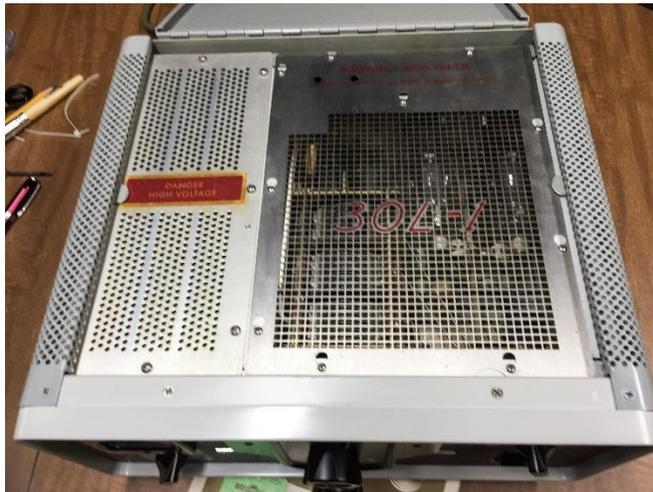
Here is a view of the 30L-1 Linear Amplifier with the cabinet cover door open. Compare this with the above interior picture and see both the Power Supply (left) and RF Compartment (right) covers in place. See also the unique punch pattern for the RF Cover that allows the model number to be silk screened in the active area of ventilation holes. The 30L-1 is an impressive mechanical design. That and the electrical design have withstood the test of time.
