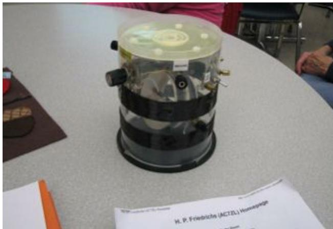
Photo 1: WB9RQR's CD-ROM-based crystal radio based on the AC7ZL design.
