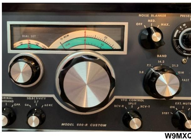
The Frequency Determination Controls on the Swan 600-R Custom Receiver – Typical if the 600-T, 600-R Standard, and the 600-R Custom.
