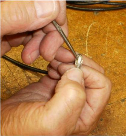
OK, it was now time to solder the coax to the tubing prior to cable-tying it to the mast. Because of the required length of the shield and the center-conductor separated by the mast, I decided to pull the center-conductor out of the braiding. If you haven't seen it done, all that is needed is a sharp tool. Start by putting a sharp bend in the coax at the point where the jacket is removed;
