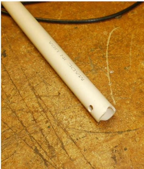
Now I needed some type of mast I could extend out the sunroof of the vehicle. Again, my shop didn't let me down. I found a piece of 7/8" OD thin wall PVC pipe and cut it to 25" in length. At the top end I used a half-round file to make a concaved spot to accommodate the tubing. Then I drilled a ¼" hole, all the way through, below and perpendicular to the concave for a cable tie to secure the top of the tubing to the mast.
