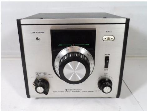
At the left, top picture, is a front panel view of the VFO-5SS Remote VFO. The VFO takes its power from the host TS-511S transceiver. Note there is a crystal socket at the upper right-hand corner and an associated crystal/VFO switch below it. The VFO-5SS could use a crystal for a single frequency location, such as a net. This was much more important in a day when free running VFO oscillators could not approach crystal stability like the PLL circuits of today.
