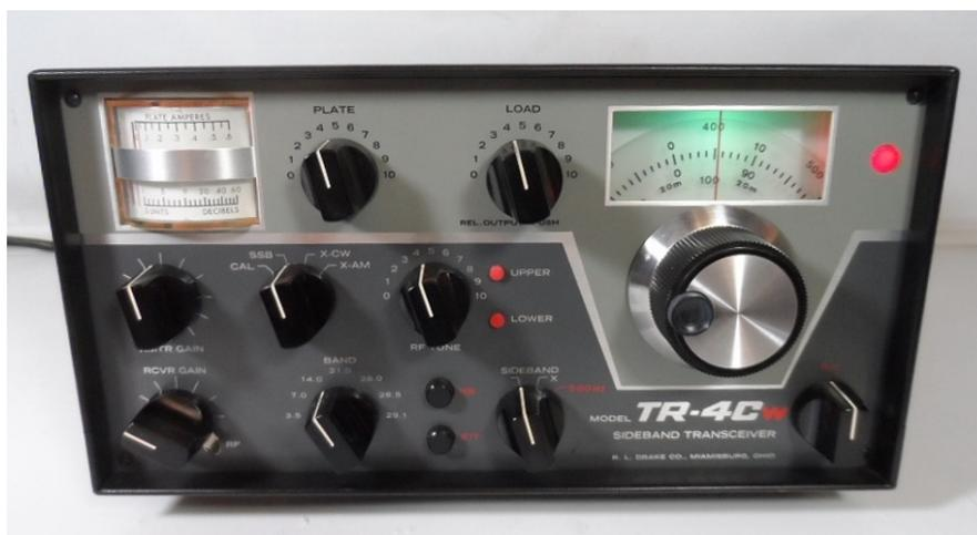
**Drake TR-4CW/RIT HF (80-10 Meters) SSB/AM/CW Transceiver**
