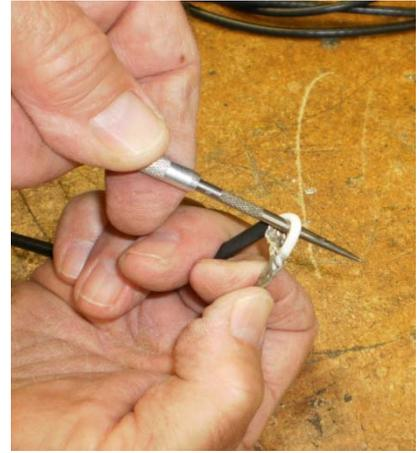
poke around and gently separate the braiding. Then put the tool between the center conductor and the braiding, push through, and slide the center conductor out.
