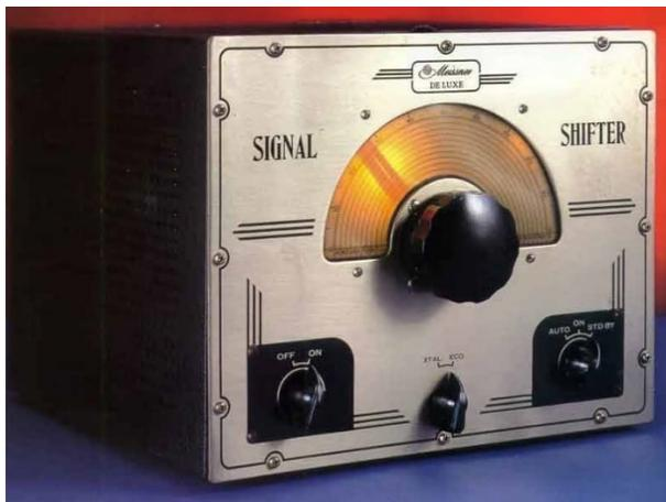
This picture is typical of the Variation 2 product under models 9-1077, 9-1078, and 9-1080. These dated from 1943 and through World War II. This little Transmitter/Exciter produced 7.5 watts output using ham band and general coverage (HF) RF coils. It was intended to run alone or with the 150-B Amplifier that had a complete audio circuit and modulator. Although low in power, the Signal Shifter could operate barefoot.
