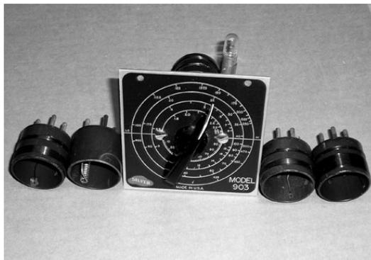
**The McMurdo Silver Model 903 Absorption Wave Meter and 4 of the 6 coils used to indicate the frequency of the monitored RF field**
