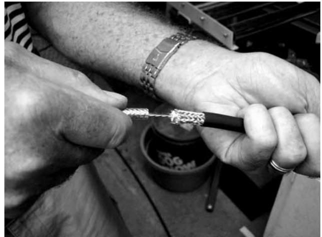
Now cut through the insulation to the conductor. Now slide the insulation off the conductor and you are ready to assemble the coax connector onto the cable and solder the shield (if copper) to the housing.
