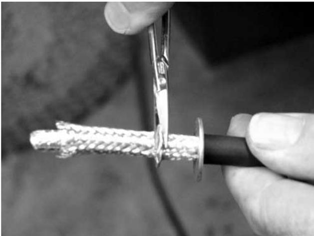
Use manicure scissors to trim around the shield at the base of the flange and then slide off the excess shield.
