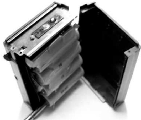
**After unsoldering the original pack and installing the replacement pack (and temperature sensor) the case is easily reassembled.**
