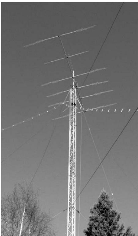
Notice the open wire folded dipole made by Ray and also suspended from the tower.
