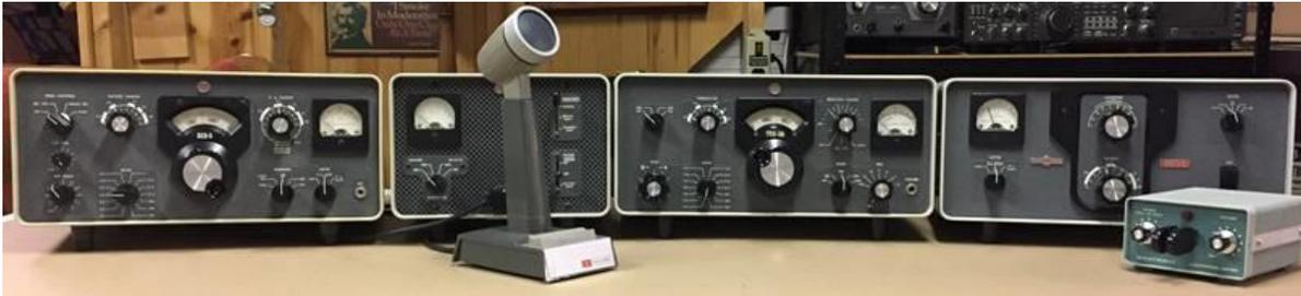
**Collins 32S-3 Transmitter, 312B-4 Console, 75S-3B Receiver, 30L-1 Linear Amplifier
