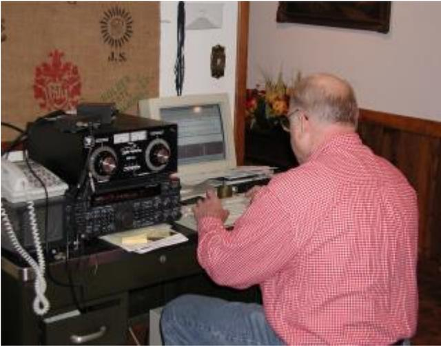
Here we see Kent Christiansen, N9WH, in 2002 making his first PSK-31 contact with his new Rigblaster on 20 meters. Kent was getting out using his Kenwood 950SDX transceiver, Nye Viking antenna tuner and a 500+ foot "loop" antenna strung "around" the back yard.
