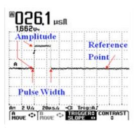
or voltage, of 1.662 volts. Digital pulses usually have a well-defined shape, e.g., rectangular or triangular, but in reality they may have various shapes at random intervals. Electrical noise would be a good example.
