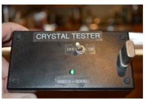
It is a one transistor Colpitts oscillator. The oscillator output is fed to a second transistor that is simply a switch to turn on the green LED, indicating your crystal is properly oscillating. I have had a HC-6 crystal socket for about 40 years in one of my junk boxes, so I dug that out (took hours to find it---) and used it for this application. With any other crystal style, I will simply plug in some short test leads with an alligator clip on their ends.
