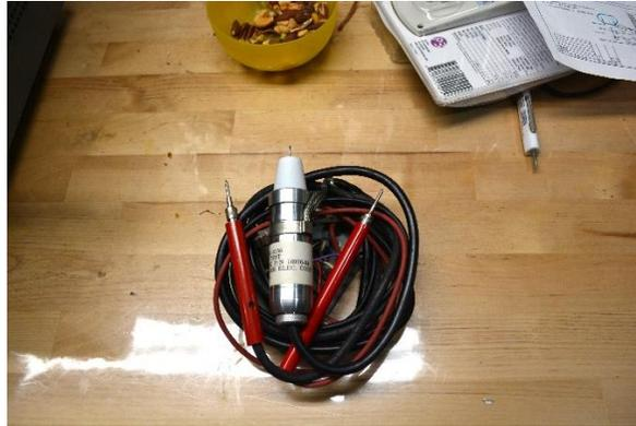
Two working RF voltmeters aren't enough, so here is the third, a Hewlett Packard 410C. When bought it was a train wreck, now is working fine but still needs AC voltage to be calibrated.
