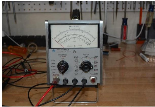
This item was missing the bottom cover, the AC plug on the back was one that no cords can now be found to match the socket, and still used one vacuum tube, the rest all solid state.
