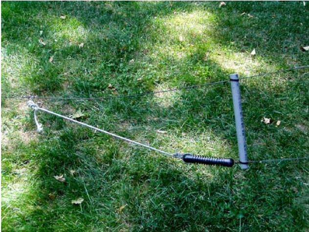
The longest spreader is used at the end of the 20 meter fan and the end insulator is secured up to the supporting 80/40 trap dipole.
