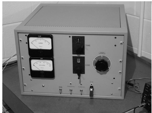
I can drive the amp to 1300-1400 watts output, and the plate transformer never even gets warm.
