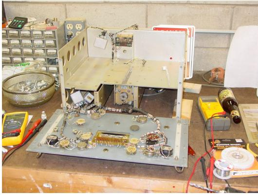
Please note the empty “fuel” container on the right side of this picture. The capacitors were all replaced, and several out of spec resistors. Then the RF deck gear train was 100% disassembled and all of the 46 year old grease removed one gear at a time. The gear train was re-assembled and aligned, a project that you do not want to do every night of the week. It is very demanding and requires perfection, for a proper function receiver.
