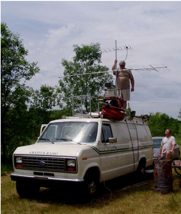
**Ken Boston (W9GA) was busy attaching the 2 meter and 70 cm antenna to the OZARES communications van mast under the supervision of Todd Sprinkmann (KC9BQA)**
