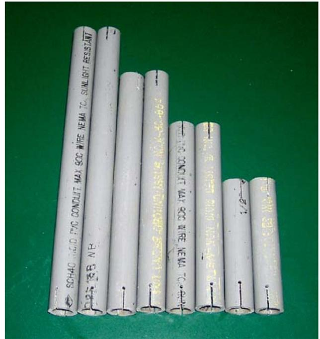
The conduit was cut into 4”, 6”, 8” and 10” lengths with the shorter spacers to be used nearest the center balun.
