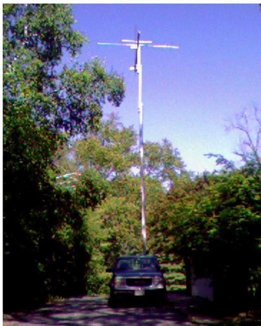
Next, I mounted it in the truck with an attached rotor and a 2 meter and a 440 beam antenna. Additionally, I added an aluminum angle for mounting omni directional antennas that I would build in the future. By this time, I was pretty far along and needed a reality check and some good input. I called Tom Ruhlmann, W9IPR, and asked if I could show him what I was working on. He gave me some good ideas and encouragement. I am working on one of his ideas
