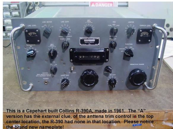
This is a Capehart built Collins R-390A, made in 1961. The "A" version has the external clue, of the antenna trim control in the top center location, the R-390 had none in that location. Please notice the brand new nameplate!
