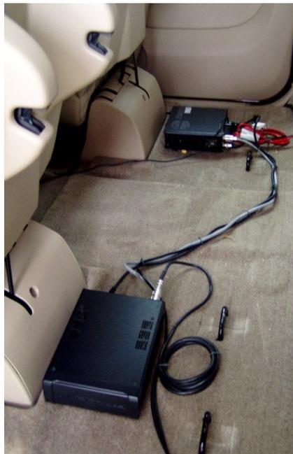
The previous vehicle had a bench rear seat with plenty of room for the transceiver and antenna tuner however in this vehicle, with separate "captain's" seats in the rear the units had to be located separately . A floor mat will cover the interconnecting cables.
