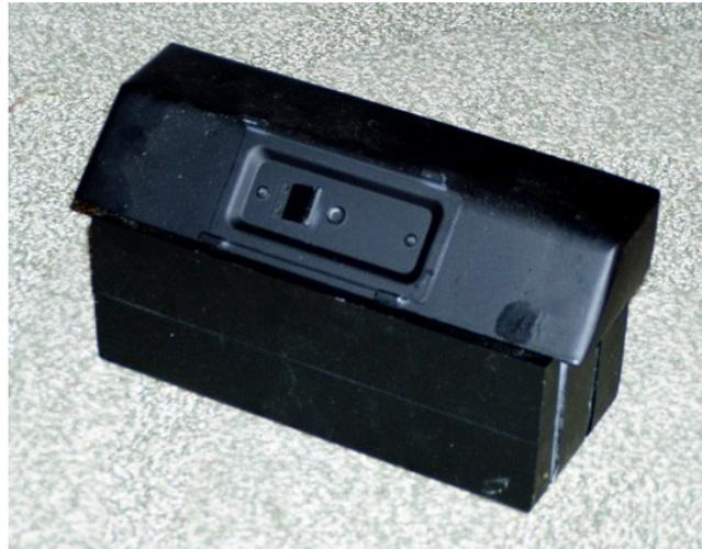
A solution for the control head mount was to cut a wood block to place in the drink holder position and reposition the drink holder to the rear of the compartment.
