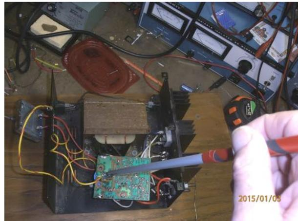
The completed rod with tip probe and grounding wire/clip. To use, simply attach the alligator clip to chassis and touch the connected end probe to the filter capacitor +..
