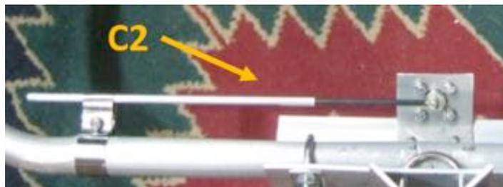
The center of the Gamma match (the brass rod) is connected to the center of the SO-239 connector and the tube is spaced from the lawn chair leg, I mean antenna element, in such a way as to allow adjustment for tuning.
