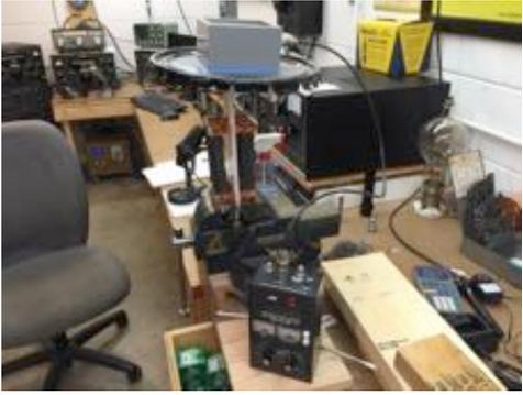
SWR checked from 1:1 up to 1.4 to 1 at 30 MHz, so the final assembly took place, resulting in the completed dummy load.
