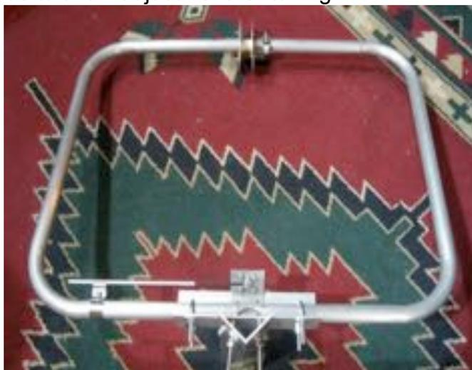
With the fabrication of a mounting bracket the completed antenna looked like this:
