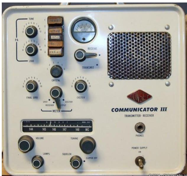
Gonset Communicator III. 2M AM Transceiver (actually, more properly called a Transmitter – Receiver as there were no common components other than the power supply and cabinet.
