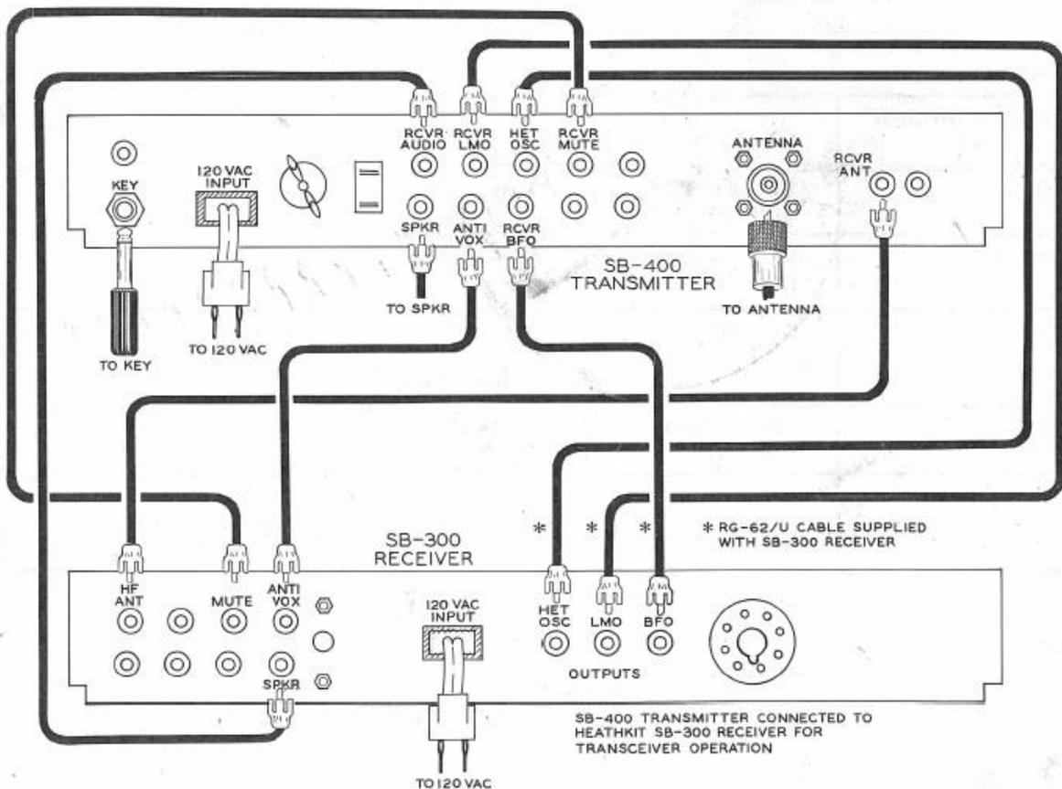
**Heathkit SB-300 Receiver and SB-400 Transmitter
