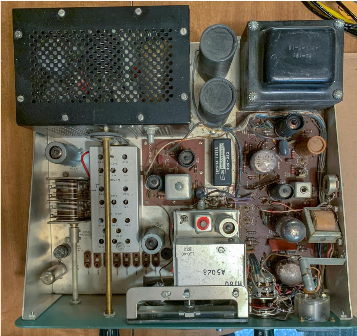
**Top Chassis View of the SB-401 Transmitter – Outer Cabinet Removed.
