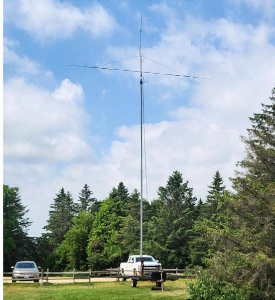
**40-meter phone rotatable dipole.**
