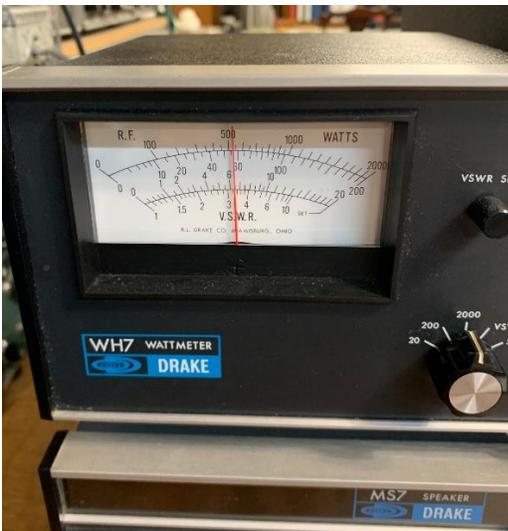
This is the Drake WH7 Wattmeter showing 520 watts output. At 1,008 watts input this shows a plate efficiency of about 52%. That is acceptable for this amplifier operating in class AB1.
