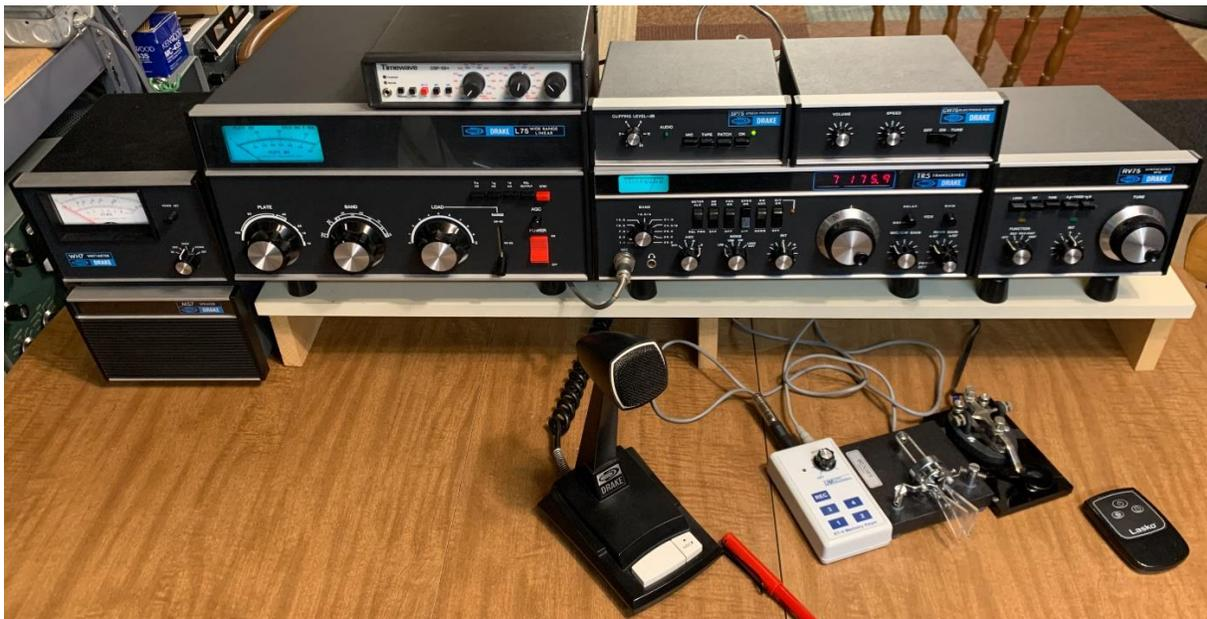
**Front and Center – Drake L75 Linear Amplifier, Drake TR5 HF Transceiver, Drake RV75 Digital Remote VFO with other Accessories.**
