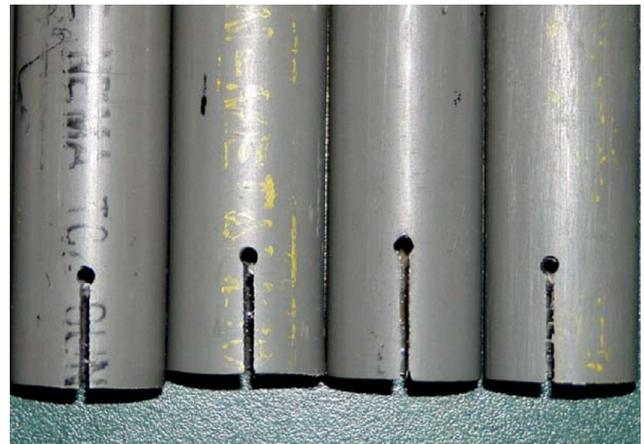
A thin 1” long slit was then cut in both ends of the spreaders and a small hole was drilled at the bottom of each of the slits. The hole should be about the same size as the antenna wire. The slit allows the antenna wire to be pulled into spreader. A properly sized hole will allow the spreader to clamp the antenna wire in place.
