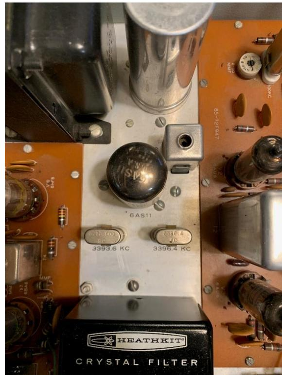
**This is the BFO Oscillator area of the SB-300 Receiver.**
