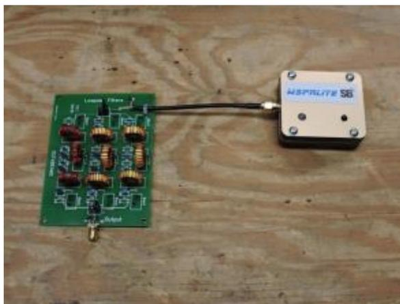
The device is called the WSPRlite (<http://www.sotabeams.co.uk/wsprlite>). It's a 200 mW WSPR transmitter that supports the 20m and 30m bands, and with the added Low Pass Filter kit it can operate on the 40m, 80m, and 160m bands. The WSPRlite transmitter comes assembled in a 2"x2"x0.75" enclosure. The only interfaces are a micro USB port for power and configuration, an SMA connector for an antenna, and a button to start transmitting.
