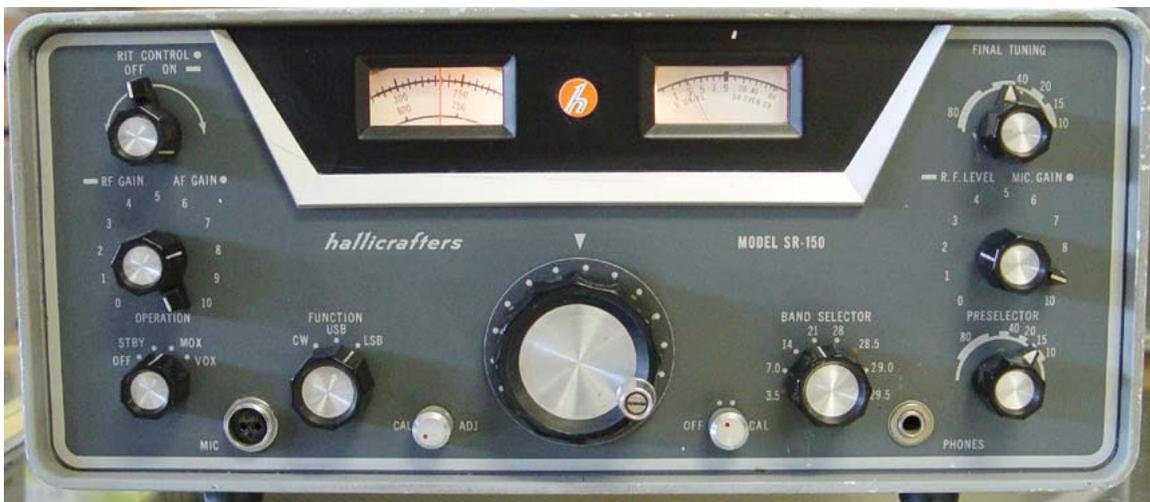
The front panel size of the SR-150 and the SR-400 were identical but complexity was increased in the later model. The addition of a very effective Noise Blanker, separate CW Filter, and Notch
