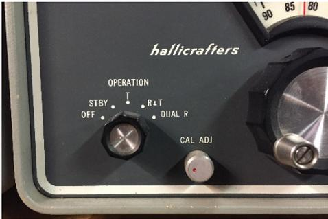
Check the OPERATION switch in the picture at the left. There are five modes for the HA-20 (for this list just below, R = Receive and T = Transmit):
