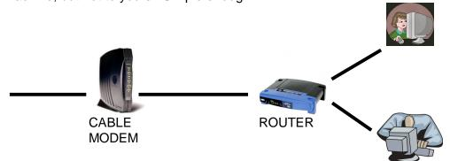
The black lines in the diagram above represent cable connections, with cable coming into the cable modem from your Internet Service Provider, then going to the router, then to your wife's computer and to yours. The cables are connected to both computers. On the other hand, your computer never sees a packet of information addressed to your wife's computer. The router routes it to hers, but not to yours.
