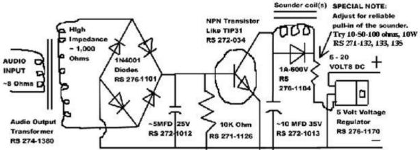
This simple circuit will allow you to take any audio signal such as the output of a receiver or code practice oscillator and use it to drive a sounder. You will need to select the value of the noted resistor to be as large as possible while still providing reliable pull-in of the sounder. This will avoid heating of the sounder coils and prolong its life.
