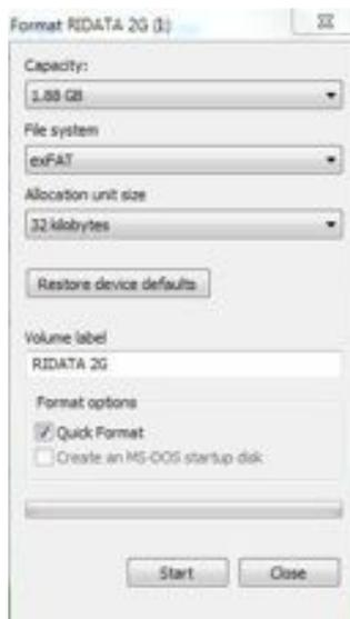
If you have a new flash drive (or an old one that you wish to redo), plug it into a USB port, right click it in My Computer and select format, as shown to the left. Select exFAT as shown, Quick Format, click Start and the drive will be prepared in a couple of seconds. **NOTE THAT THIS PROCEDURE WILL DELETE EVERYTHING ON THE FLASH DRIVE.** If you have files that you want to save, copy them first to your computer, then back when you have finished formatting the flash drive.
