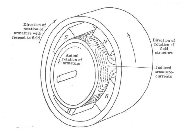
THE ROTATING SPEED OF THE ROTOR IS LESS THAN THE SYNCHRONOUS SPEED BECAUSE LIKE THE DISC, THE ROTOR CAN'T KEEP UP.
