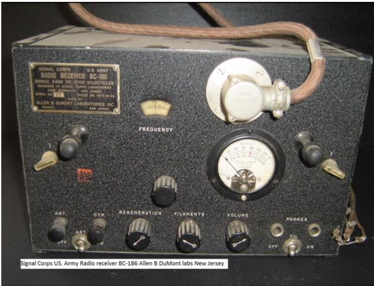
#2 Signal Corps US Army Radio receiver BC-186 Allen B DuMont labs New Jersey
