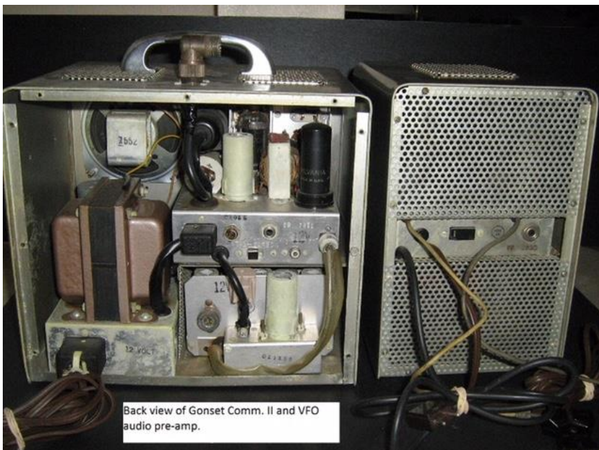
Gonset Communicator II, 2meter Transmitter-receiver on the left Gonset 2 meter VFO Audio Pre-amp on the right
