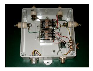
The antenna relays, connectors and terminating resistor were housed in a water tight plastic box that I got at the ORC May swapfest for \$2.00. The robust feedthrough insulators form the terminations for each side of the loops.
