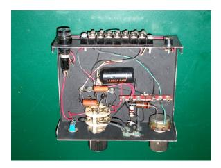
The control circuitry was made completely from the junk box using an old "A-B" switch for the control box itself.
