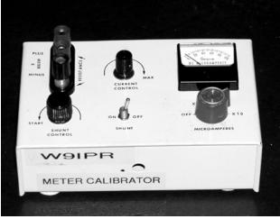
The "Meter Calibrator" using a 100 microampere standard meter with scale multipliers of X2, X5 and X10
