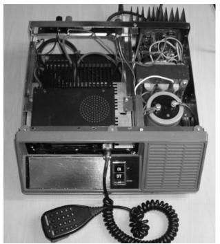
The Kenwood is installed and powered by the retained power supply and connected to the cabinets speaker
