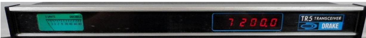
Notice that the strip is black with a silk-screened surround encircling the frequency readout window and a two-color silk-screened area to the right of the frequency readout calling out the radio's model number and the Drake name and logo. This appeared all to be covered with olive drab paint. This is critical here because I had already discovered on the PS7 panel that the silk-screened area was vulnerable to the paint remover.
