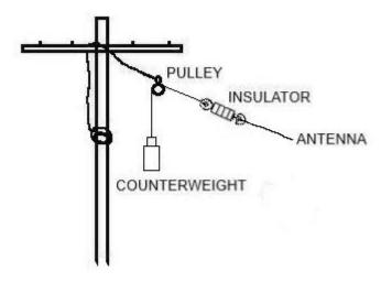
The counterweight keeps the antenna taut so there is very little "belly", and high winds, ice or snow offer no danger to the antenna's position. But, as we have seen, a falling tree will bring it down (without breaking it), until it pops back up when the tree is removed.
