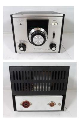
At the left, top picture, is a front panel view of the VFO-5SS Remote VFO. The VFO takes its power from the host TS-511S transceiver. Note there is a crystal socket at the upper right-hand corner and an associated crystal/VFO switch below it. The VFO-5SS could use a crystal for a single frequency location, such as a net. This was much more important in a day when free running VFO oscillators could not approach crystal stability like the PLL circuits of today.
