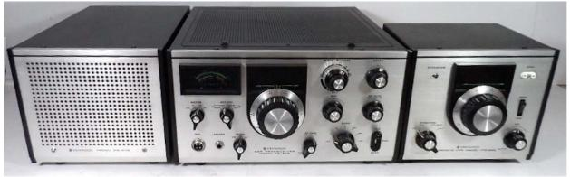
Left to Right PS-511S Power Supply, TS-511S Transceiver, VFO-5SS Remote VFO W9MXQ Photo
