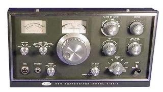
Allied Radio A-2517 HF Transceiver from 1970. This perhaps is the first Trio-Kenwood radio to be marketed in the USA. Comparing this radio with the Trio TS-510 shows them to be similar, if not identical. There was also a very nice A-2516 Receiver that would have worked well as a partner with the A-2517 shown here. The A-2515 was not designed to transceive with the A-2517, to my knowledge. These date from about 1970.
