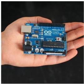
Arduino Uno microcontroller prototyping board. (photo courtesy Arduino: http://www.arduino.cc/)
