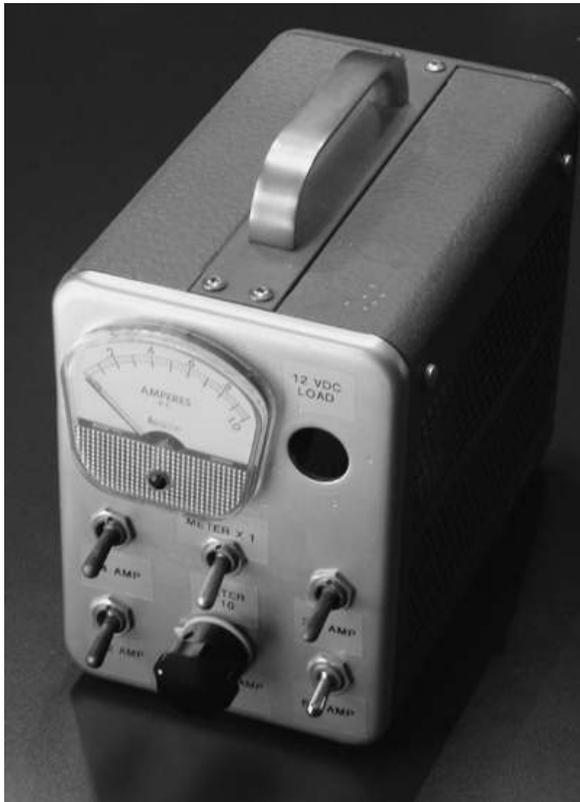
**The completed 12 VDC Resistive Load Box.**
