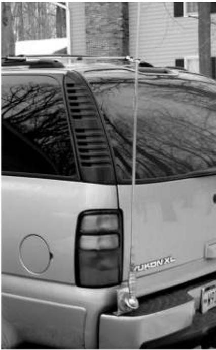
The HF antenna coax was also passed through the hatch door seal gasket and under the carpeting to the transceiver. Notice that the Hustler antenna was stabilized to the luggage rack using a stiff plastic rod (electric fence pole) and tie wraps.
