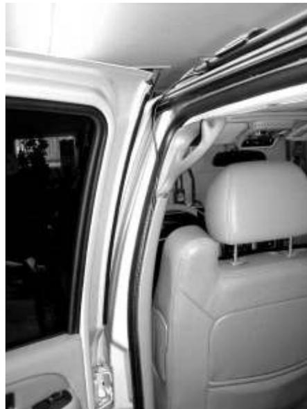
A “mag mount” UHF/VHF antenna was used as in the past and the coax was passed through the door and along side the door seal gaskets. Should the coax eventually be damaged just replace it. It’s a lot better than cutting a hole in the vehicle.
