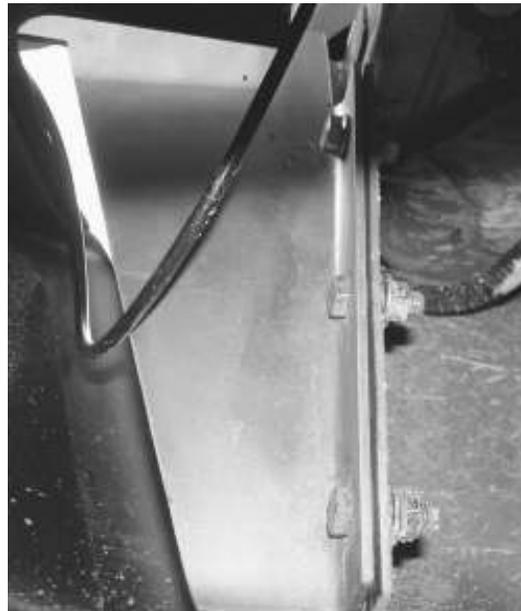
The lower portion of the mount that clamps to a fender flange is shown here from below the vehicle.
