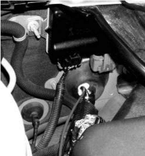
The power leads from the battery were threaded along a main wiring harness that already passed through the firewall using a blunted clothes hanger. I was especially careful to avoid damage to any of the existing wires in the factory harness.
