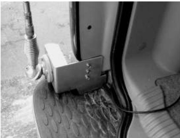
A special bracket was fabricated to mount the HF antenna ball mount. Shown is the upper portion. Note the mount rests on the bumper. This upper portion is secured with 3 metal screws to the doorframe to prevent any lateral motion of the mount. So OK, I did drill some holes but they were small.
