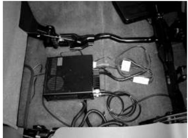
The exposed power wiring was protected with spiral "wrap around" plastic harness available at Radio Shack. Power connections were made using Anderson Powerpole connectors. A ferrite core was placed around the power cable "just in case".
