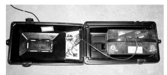
With the cover opened the internal wiring behind the panel is shown as is a storage area in front of the battery. Note the ventilation slots in the cover to allow for venting of any hydrogen gas that could be generated during charging.
