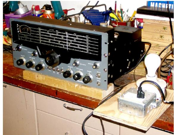
Once it is determined the suspect load has no short to chassis or other fault drawing high current the test switch can be turned “ON”, shorting out the “dim lamp” and applying full voltage to the load being tested.
