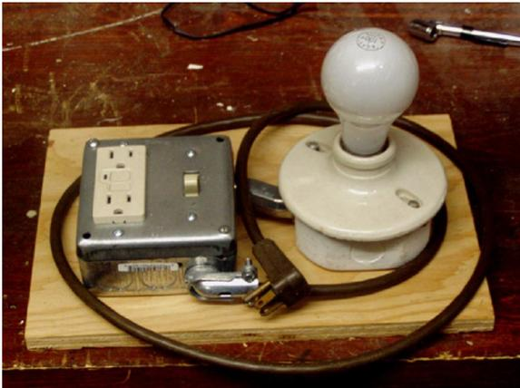
Another approach is to build and use a so called “dim light” tester. The parts are readily available in many junk boxes or at the local hardware store at small expense.
