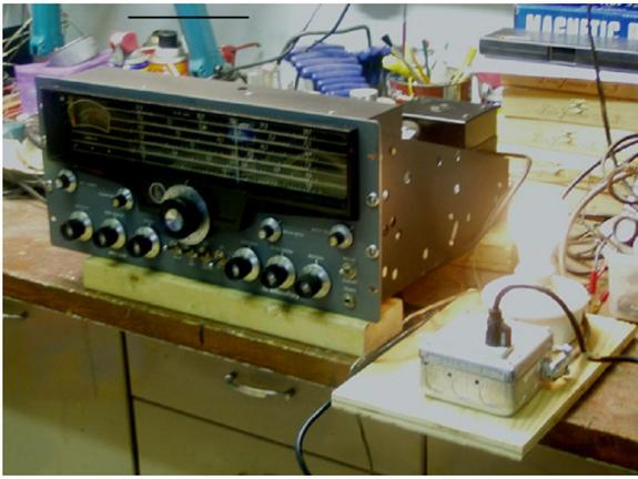
Note that when this restored vintage receiver is plugged in to the GFI receptacle of the “dim lamp” tester the receiver lamps and test lamp glows dim indicating the line voltage is being divided between the receiver and the “dim lamp”.
