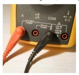
high and hopefully you're using a meter which is fused. If not, it could blow up or at minimum fry the insides. Naturally, the severity is dependent on the power you're working with.
