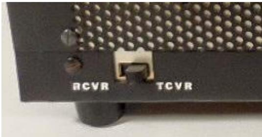
My Drake collection includes an early TR-4, a TR-4C, and a TR-4Cw-RIT. In every case, the switch pictured to the left is present on the left-lower-rear side of the cabinet. It switches the radio from using the Internal Transceiver (TCVR) or an External Receiver (RCVR).
