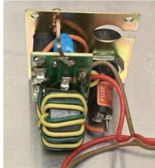
**Closeup of the Access Panel that Mounts to the Back Panel of the IC-751A.**
