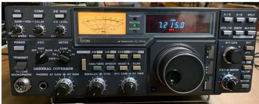
This relatively early all solid-state radio brought excellent receive audio, transmit audio, receiver AGC, and QRM Control as we have come to expect from modern radios – but remember that this was the 1980's. This radio basic design (original IC-751) is now over 40- years old.
