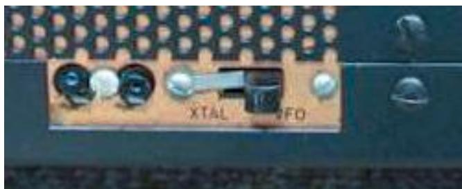
This is the Slide Switch on the Drake R-4B Receiver at AC9CD. It is located on the lower rear left side of the radio. Note the Slide Switch with the Tab installed to keep the switch in the "VFO" position.
