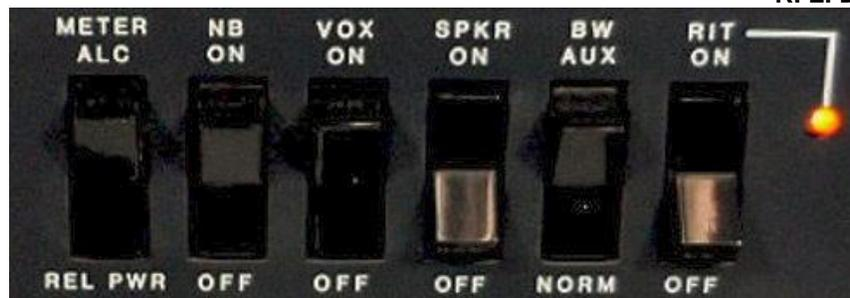
**Rocker Actuator Equipped Slide Switches on the Drake TR5 Transceiver in 1981**
