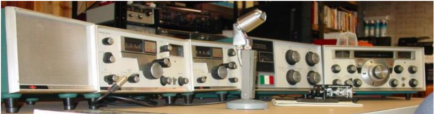
Left to Right are the National NCX-A AC Power Supply/Speaker, the NCX-5 HF Transceiver, the VX-501 External VFO, the NCL-2000 Linear Amplifier, and the HRO-500 Receiver. The HRO-500 here is acting as a second receiver with the NCX-5, when desired.
