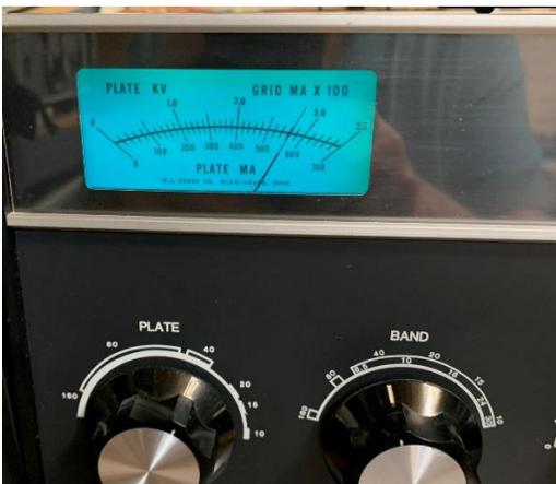
TR5 running 70-watts showing 2,800 DC Volts on the plate of the 3-500z. Plate voltage at key up (no output power) is about 3,100 volts.
