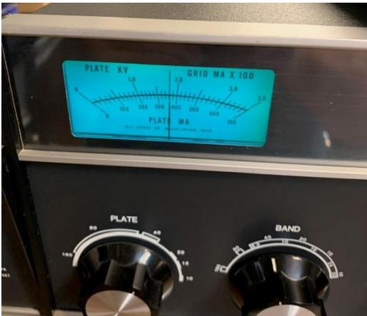
TR5 running 70-watts showing 360 mA of plate current on the 3-500z.
