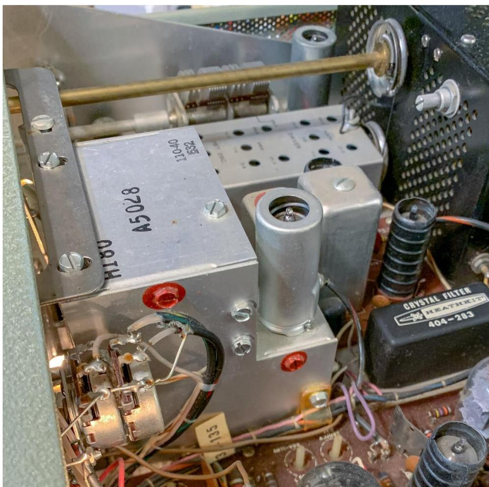
**SB-401 LMO – installed in place. Note red paint to indicate “Factory Sealed.”
