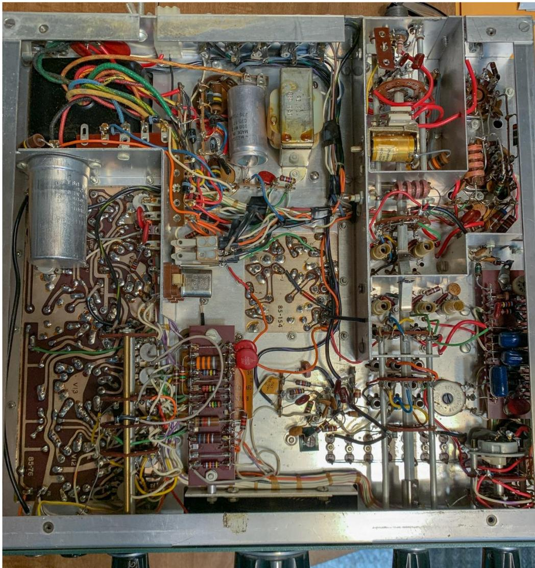
**Bottom Chassis View of the SB-401 Transmitter – Outer Cabinet Removed.
