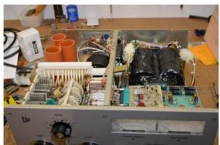
worked as normal. I let it go at 1700 VDC for another 24 hours, prior to going any further. The normal voltages for this amp are 1500 VDC in CW and 2200 VDC in SSB. I do have four "DANGER HIGH VOLTAGE" signs that I set up around this kind of situation, then I barricade my work shop with chairs so no other family member can venture into that zone. Seems to work pretty well!
